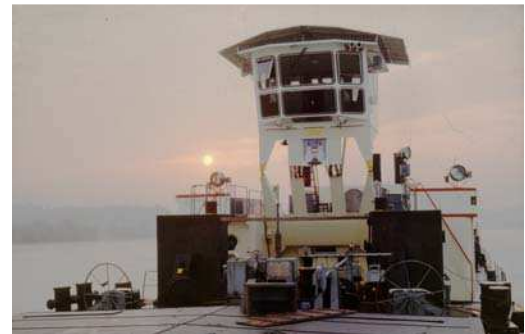
Figure 42 Lifting wheelhouse mpv Ybbs
